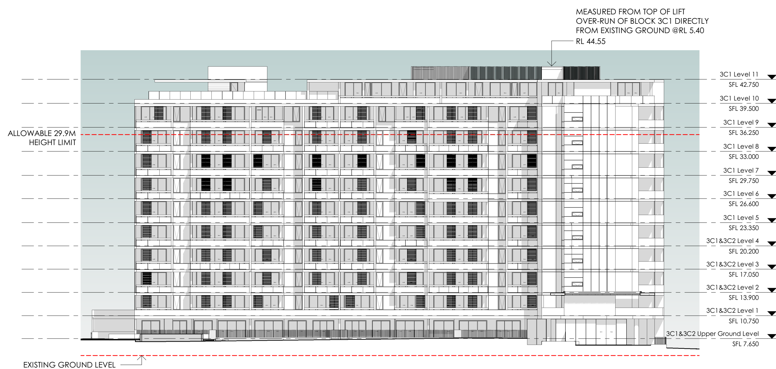
3 Block 3C1 - North Internal Courtyard
